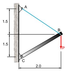
Bar AB has a cross-section of .25"x4" and CD is .60"x4". With a load of 2-k at the end, what is the axial stress in link AB and CD. Note: The units of "k" means 1000 lbs, often referred to as "kips". Units: K, ft.
