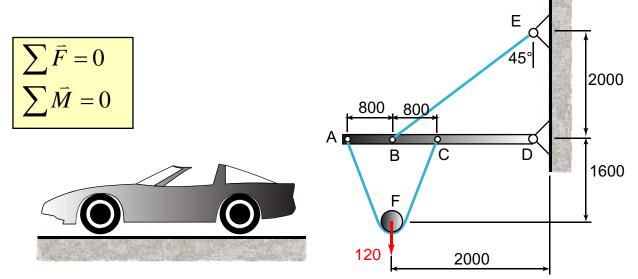
Determine the reactions at D and the tension in BE. The wire connected at A and C is continuous. Units: N, mm.
