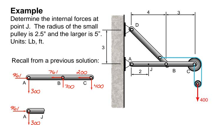
Determine the internal forces at point J due to P=500 lb and M=700 ft-lb. Units: Lb, ft.
