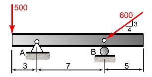
Determine the reactions at A and B. Units: Lb, ft.
