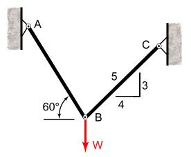
A strut and cable assembly ABC supports a vertical load P= 1.8 kN. The cable has an effective cross-sectional area of 12000 sq. mm and the strut has an area of 25000 sq. mm. Calculate the normal stress in the cable and strut, and indicate whether they are in tension or compression. Units: m
