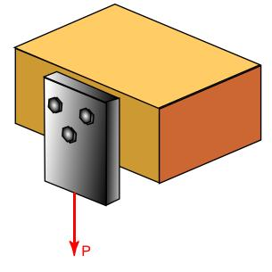
A 5/8" bolt is used at C to connect to the wooden member BC that has a cross-sectional area of 5.25 in<sup>2</sup>. Knowing that the utimate shearing stress is 58 ksi for the bolt and that the ultimate normal stress is 7.2 ksi for member BC, determine the allowable load P if an overall factor of safety of 3.0 is desired. Units: Kips, in.
