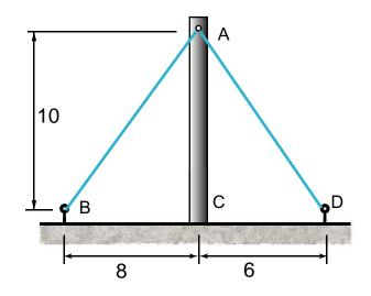
Determine the reactions at supports A and B. Units: Lb, ft.
